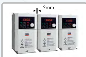
Side-by-side Installation (2mm between drives)
