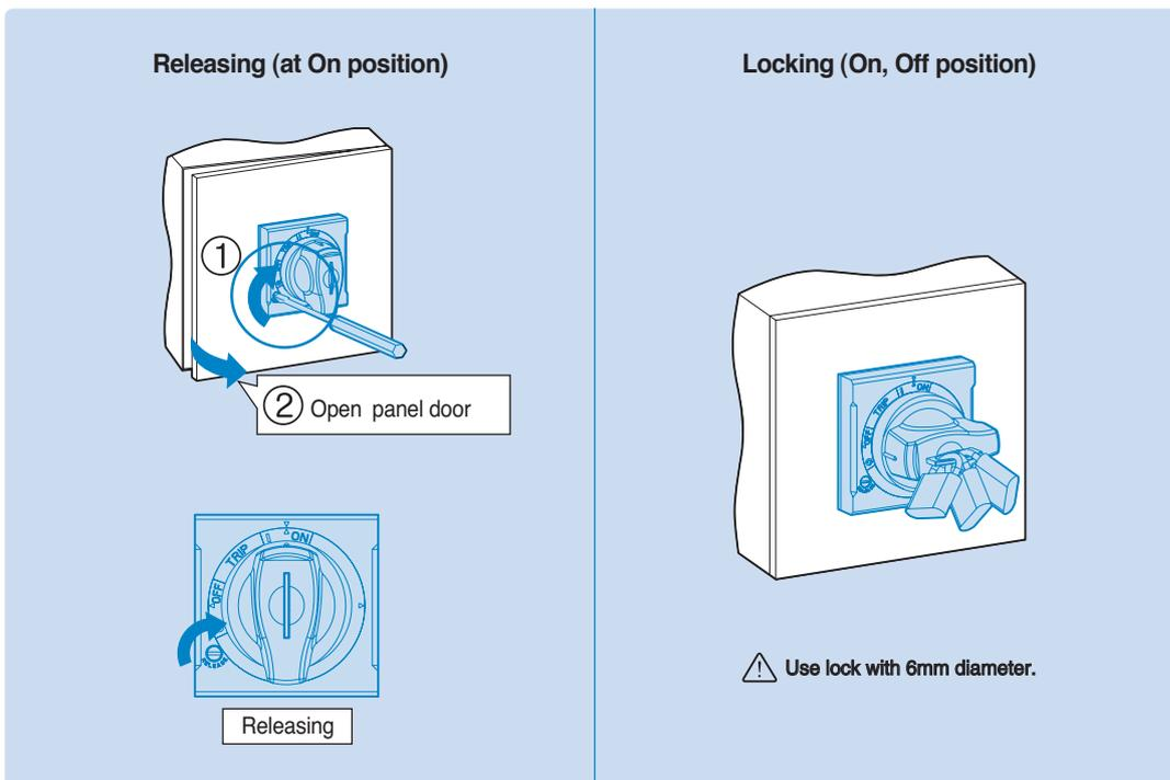
Note : In case of EH100/125/250 Semi Type, it is possible to lock E-handle only in the condition of OFF.
