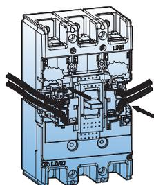
It consists of one auxiliary switch (AX) and one alarm switch (AL) in a body to connect into the same position of the breaker.
