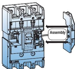
The undervoltage release automatically opens a circuit breaker when voltage drops to a value ranging between 20% to 70% of the line voltage. The operation is instantaneous, and after tripping, the circuit breaker cannot be re-closed again until the voltage returns to 85% of line voltage.
