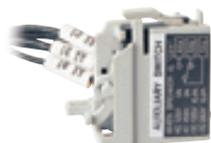
Auxiliary switch is for applications requiring remote "On" and "Off" indication. Each switch contains two contacts having a common connection. One is open and the other closed when the circuit breaker is open, and viceversa.
